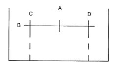
e. Measure the height of the bottom legs crossmembers and subtract ½ from that measurement. Transfer these measurements to your leg centerlines and call them E, F, G, and H.
